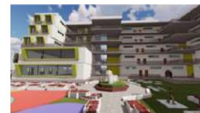
3. Staggered cantilever flooring to create shading in the floors below and central open space for leisure
