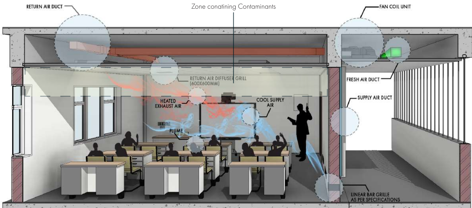
Figure 11: Displacement Ventilation Schematic
